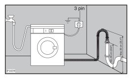
The drain hose may be extended to a maximum of 4 metres. An additional drain hose and joining piece is available from your local Service Force Centre.
